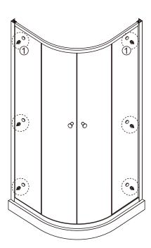
Follow the indications on wall profiles to locate the drilling holes
