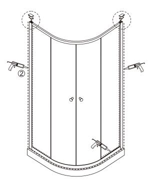
The sealant should be applied to the outside edge.
